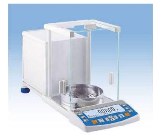
The **XA.R2** series represents a new standard level for analytical balances. They feature a new, readable LCD display which allows a clearer presentation of the weighing result. Besides, the display has a new text information line allowing to show additional messages and data, e.g. product name or tare value.
